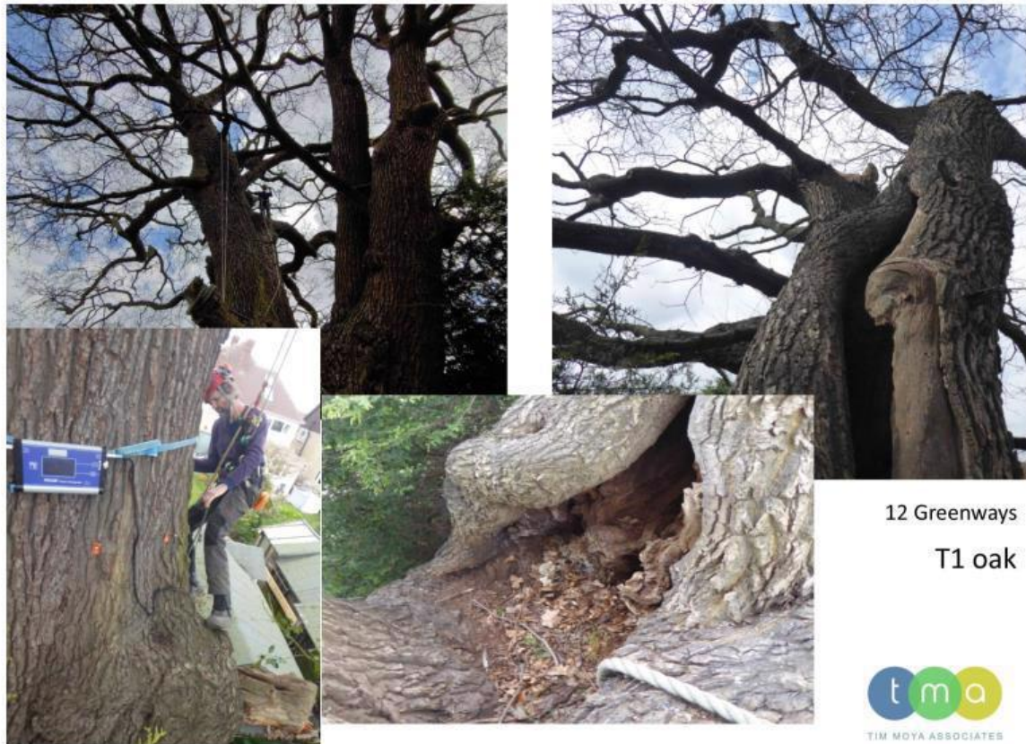
Climbing inspection of crown: Clockwise from the top left, arborist Jim Curry in the tree, cavity in limb to the west, base of same cavity, Jim Curry undertaking PicUS test @ approximately 5.5m
